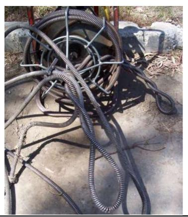
The damage to this snake cable was caused completely from misuse. THE EQUIPMENT PROTECTION PLAN does NOT COVER misuse.
